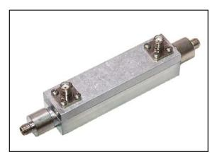
The Model C1-A55 single directional coupler covers applications in the 698-2800 MHz frequency range with high power, low insertion loss, very high directivity, and excellent PIM performance that is inherent with airline coaxial deisgn and construction. The unit is designed for mode free performance up to 19 GHz. The unique multisection suspended slabline construction yields the lowest possible insertion loss with high power handling.
