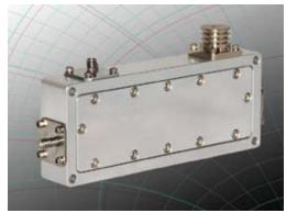
The Model C1-A59 directional coupler operates over the full frequency range of 400-2900 MHz. The nominal coupling value is 6 dB and the flatness is held within +/- 0.5 dB over more than 80 % of the frequency band. The unit features excellent PIM performance and offers directivity of better than 20 dB over frequency range. The unique "n" multisection design is ideal for
