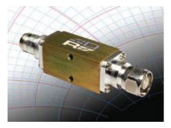
Model DC-A22 DC Block covers wireless applications in the 1000-6500 MHz band. Available with N male and N female connectors, RF power ratings of 500 watts (3.0 kW peak) and a breakdown voltage of 3.0 kV. Insertion loss is less than 0.2 dB and RL is better than 20 dB, making it ideal for antenna line applications, eliminating unwanted DC voltages in base station installations.
