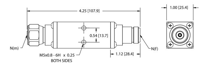
DIMENSIONS: in/mm TOLERANCE: +/- 0.03/0.8
