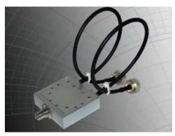
The Model HM-A05 is 1x2 divider in a high power 2way symmetrical design operating in the frequency range 700-2200 MHz. It is a resistor isolated. Wilkinson design utilizing high power resistors. The unit is provided with a type N female input connector and (2) cable outputs with DIN male connectors. Cable lengh is specified with a dash number added to the model number, (4)=4feet, (6)=6feet standard.
