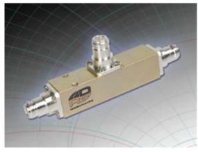
R&D unequal power dividers use a novel, patented airline structure. The fixed split ratio is maintained over a 150 to 500 MHz bandwidth with minimum ripple and insertion loss. DC is continuous through the main line, while the coupled ports is DC isolated from the main line and passes only RF power. The mechanical design has no solder joint and uses reliable, flange mount connectors with O-rings to achieve an IP65 environmental rating.
